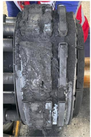
(fig.2) Heavily oxidized brake disks
