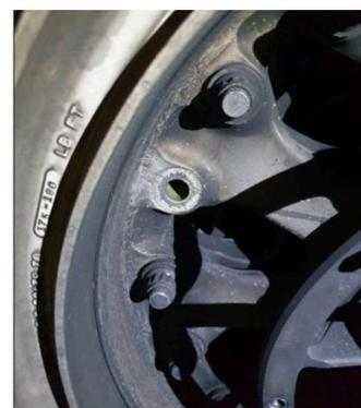
(fig.3) Example of missing tie bolt detected during a preflight walkaround (picture sent by an operator)
